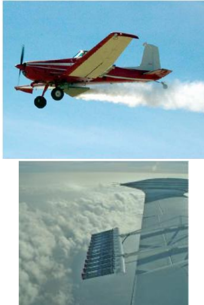
Figure 2 : Pictures of the seeder aircraft with wing mounted hygroscopic flares
